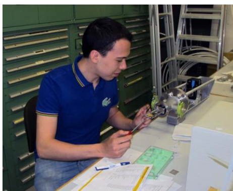
A student is mounting samples on the RBS/PIXE target holder. Some participants brought specimens from their own research projects.
