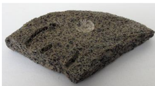
Figure 1: Experimental ceramic tile used for spot measurements. The small black temper inclusions (basaltic sand) can clearly be distinguished from the clay matrix.
